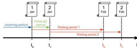
Figure 2: Timing for testing earthquake forecasts. During the **Learning Period**, modelers can deposit any data their models need to generate forecasts. After **Waiting Period 1** at time  $t_1$ , the Central Dispatcher (see Fig. 3) provides 'authorized' data to the time-dependent models. The models generate forecasts for the **Forecasting Period**. After **Waiting period 2** at time  $t_2$ , the Central Dispatcher tests the models against revised data.
